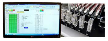
Following each critical operation in the assembly process, every sensor is tested to confirm signal output using equipment traceable to calibration certificates.
